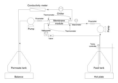
Figure 4. Schematic diagram of DCMD experiment set-up.
