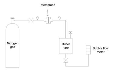
Figure 3. Schematic diagram of gas permeability measurement system.
