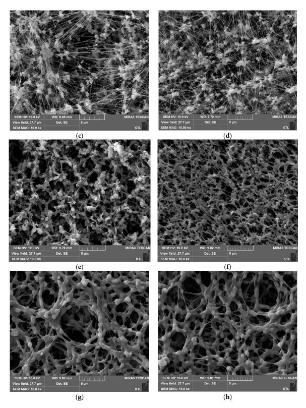
**Figure 6.** SEM images of polytetrafluoroethylene (PTFE) and PVDF membranes surfaces. The labels (**a–d**) are unpressurized FGLP, pressurized FGLP, unpressurized HVHP and pressurized HVHP, respectively. The labels (**e–h**) are unpressurized FGLP, pressurized FGLP, unpressurized FHLP and pressurized FHLP, respectively. The transmembrane pressure of membrane was set at 30 kPa.
