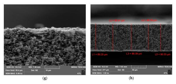
**Figure 5.** Scanning electron microscope (SEM) images for cross-sections of different polyvinylidene fluoride (PVDF) membranes. The labels (a), (b) are HVHP and (e), (f) are GVHP membranes without pressure, respectively. The labels (c), (d) are pressurized HVHP and (g), (h) are GVHP membranes at different pressure 30 kPa.
