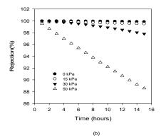
**Figure 9.** Dependence of distillate conductivity and solute rejection on time under various applied pressures  $(\Delta p)$  (**a**) distillate conductivity (**b**) solute rejection.
