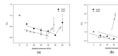
**Figure 8.** Dependence of  $J/J_0$  on applied pressure ( $\Delta p$ ) in DCMD system. (**a**) PTFE membranes (**b**) PVDF membranes.
