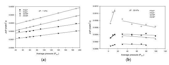
**Figure 7.** Dependence of  $J/\Delta p$  on average pressure in gas permeability experiments. (a) Low  $\Delta p$  (b) high  $\Delta p$ .
