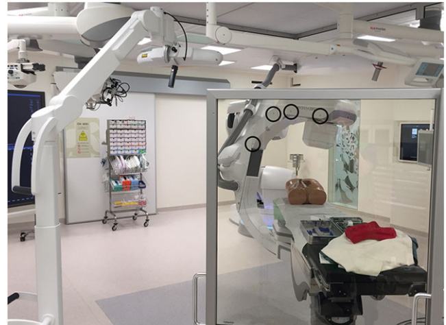
FIGURE 2 This is the starting position of the C-arm before acquiring a 3D scan. The black circles indicate the reflective calibration stickers that allow the navigation system to “see” the C-arm. The camera needs to have a clear line of sight to these stickers when starting the 3D run, otherwise the system cannot perform an automatic image registration
