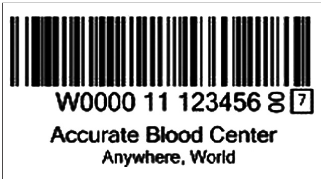
Figure 2: Format of unique donation identification barcode using ISBT 128. It has three elements: (1) the collection facility identified by the first five characters (W0000); (2) then the collection year (2011); (3) followed by a donation number assigned by the collection facility (123456). The last digit within a box is a checksum character. (Reproduced with permission from ISBT 128 An Introduction © ICCBBA Inc. http://iccbba.org/uploads/a2/6e/a26e9302a6b32cae265322947c0ef239/ISBT128introbooklet.pdf )
