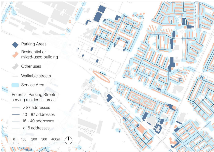
Fig. 4. Parking streets zoom-in. Streets classified by number of addresses served according to legend.
