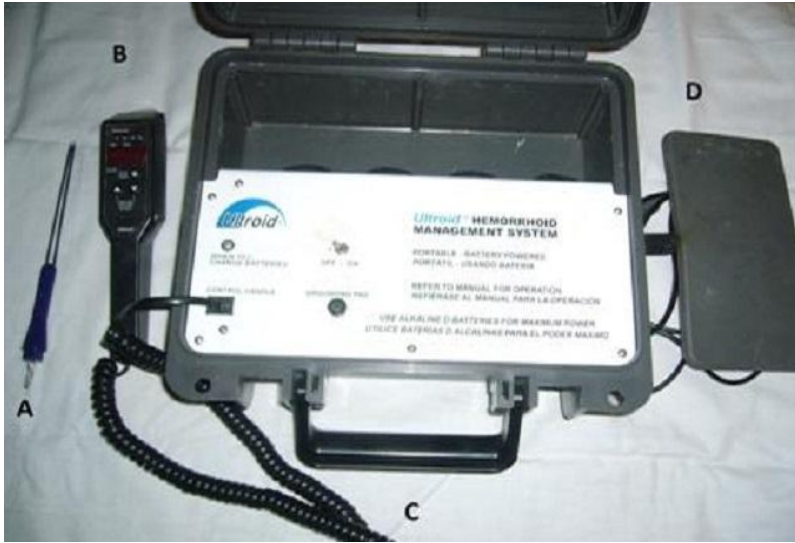
Figure 1: the electrotherapy generator components: A-disposable dual probe tip, B-probe handle, C- the electrotherapy generator, D- grounding pad
