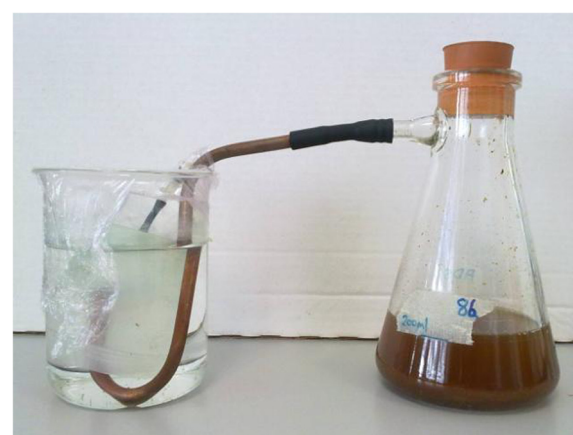
Figure 2 Conical-flask fermenter with gas collector on side-arm.
