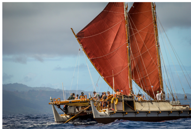
Figure 1 Photo of Hōkūle'a under traditional crab-claw sail off O'ahu, Hawai'i. She is 62 feet long and 23 feet wide, with 300 square feet of deck space for an average crew of 12 people. All food and water is stored in the hulls, where crew also sleep under the tan canvas covers. The total covered area for people to sleep—head to toe—is approximately 138 square feet. Solar panels power safety elements of maritime lights and radios. She has no engines, refrigeration, nails or screws; approximately 5 miles of rope lash her together and at least 2 miles of line make up her rigging. Copyrighted photo courtesy of Polynesian Voyaging Society and 'Ōiwi TV.
