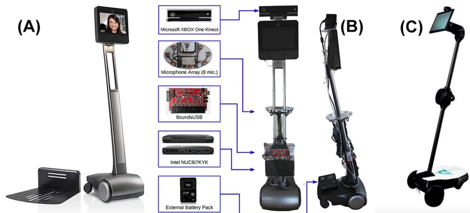
Fig. 4 Telepresence robots: (A) Beam; (B) SAM, an augmented version of Beam; (C) OhmniLabs
