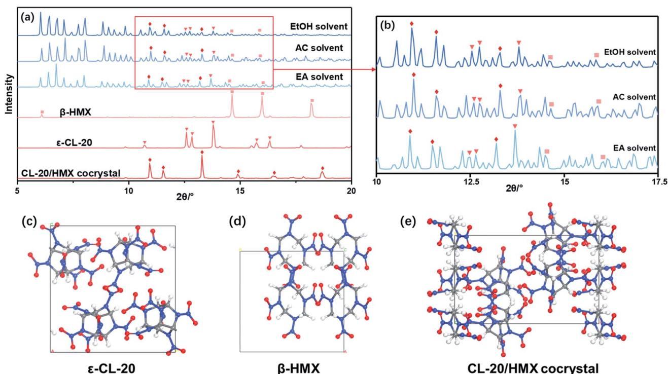
Fig. 4 (a) XRD patterns of CL-20/HMX/solvent mixtures; (b) insert of characteristic part of samples; (c–e) crystal structures of  $\epsilon$ -CL-20,  $\beta$ -HMX and CL-20/HMX cocrystal. C, H, O, and N atoms are labeled as gray, white, red, and blue, respectively.
