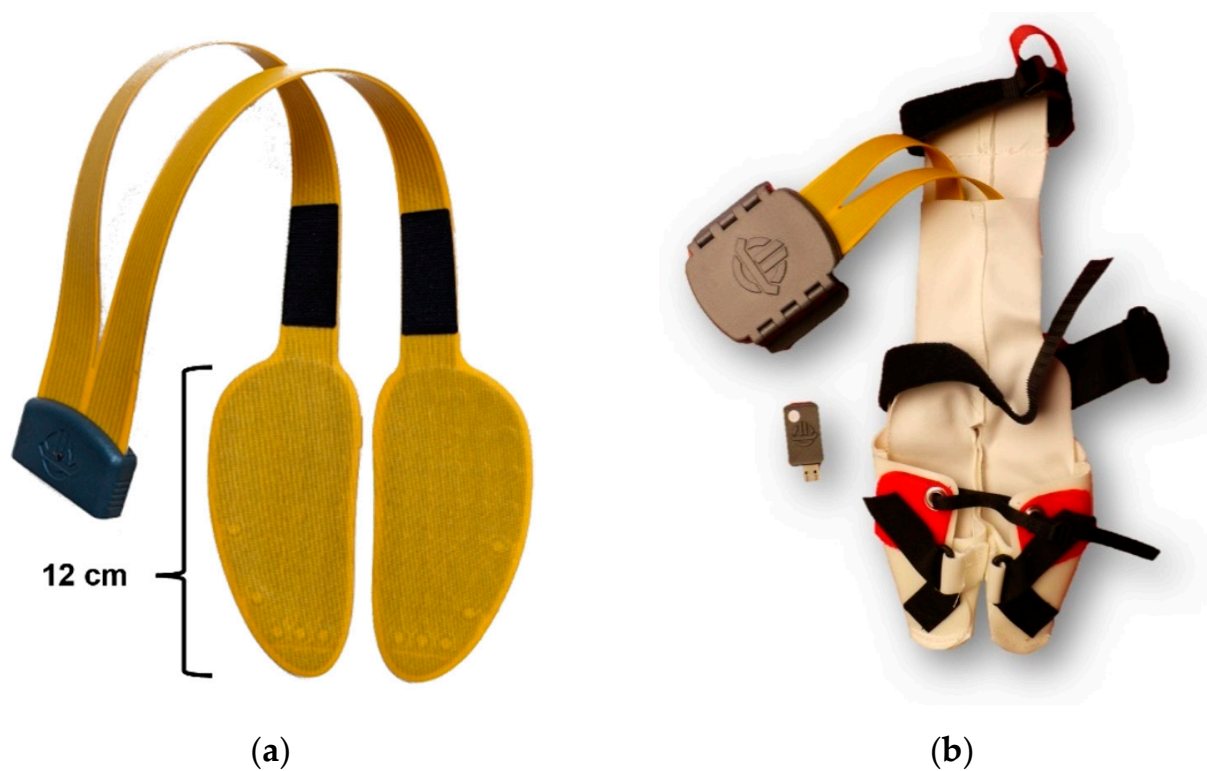
Figure 1. Sensor systems used for gait analysis in ten dairy cows: (a) paired claw-shaped pressure sensor soles; (b) textile claw shoe for attachment of the sensors.
