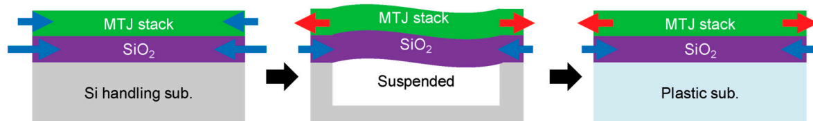
Figure 10. Schematic diagrams of transferring the MTJ stack. Adapted with permission from Ref. [91]. Copyright 2016, copyright John Wiley & Sons, Inc.
