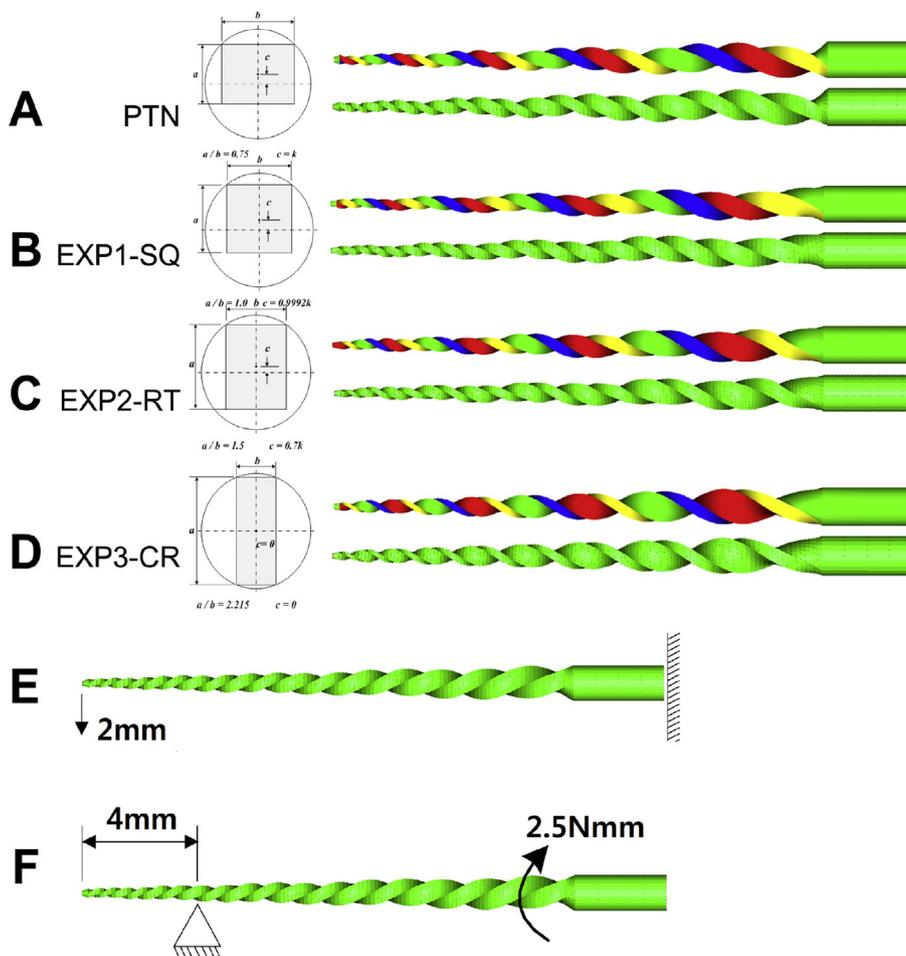
**Figure 1** Four different geometric designs were evaluated using finite element analysis. (A) ProTaper-NEXT type design (PTN); aspect ratio = 0.75, off-center =  $k$ . (B) Square (EXP1-SQ); aspect ratio = 1.00, off-center =  $0.9992k$ . (C) Rectangle (EXP2-RT); aspect ratio = 1.50, off-center =  $0.7k$ . (D) Centered-rectangle (EXP3-CR); aspect ratio = 2.215, off-center = 0. (E) Simulated flexural stiffness test. (F) Simulated torsional stiffness test.
