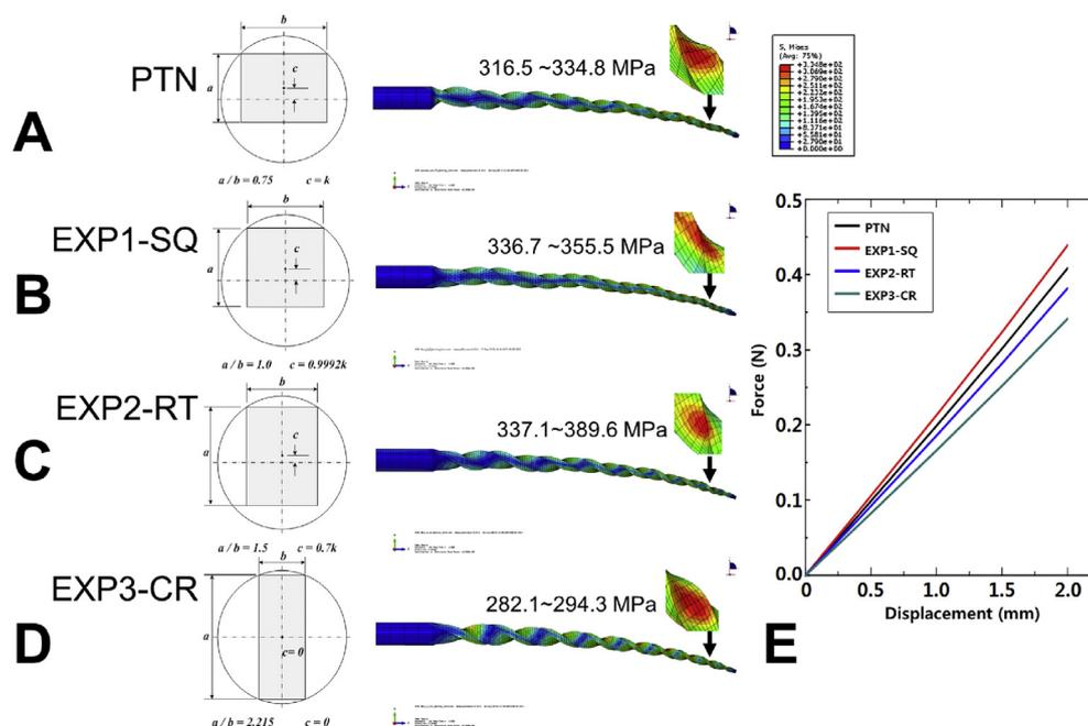
**Figure 2** Comparison of stress distribution and calculated bending stiffness of the four instrument models. (A–D) Maximum stresses were concentrated at the 3.2 mm level from the tip (arrow indicated). The ProTaper-NEXT type design (PTN) model had lower stress generation than other off-centered models, while the centered-rectangle (EXP3-CR) model had the least stress. (E) The PTN model showed less bending stiffness than the square (EXP1-SQ) model.
