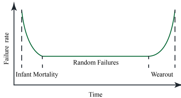
Figure 2. Failure rate "Bathtub curve".
