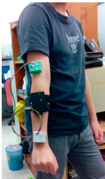
Figure 1. Implemented two-channel wireless IMU system mounted on the upper extremity of a healthy adult.
