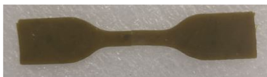
Figure 1. Exemplary ENR/quercetin2/silica15 sample (type 2 according to ISO 37 standard) dedicated to mechanical test.
