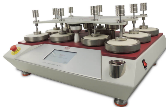
Figure 1. Martindale Abrasion and Pilling Tester TF210 [33].
