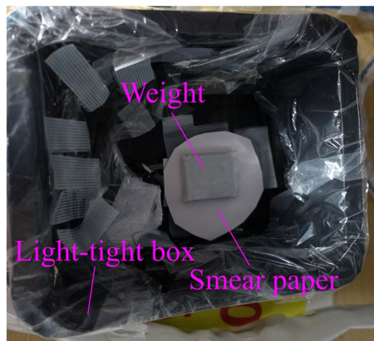
Figure 17. Photo of measurement of smear papers: Top view. The alpha particle imaging detector was placed under the smear paper.
