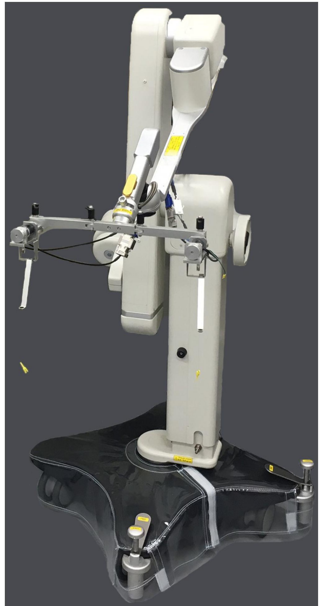
FIGURE 1 Developed microsurgery-assist robot. The developed robot composed of the arm (Uni ARM; Mitaka Kohki) and winding parts
