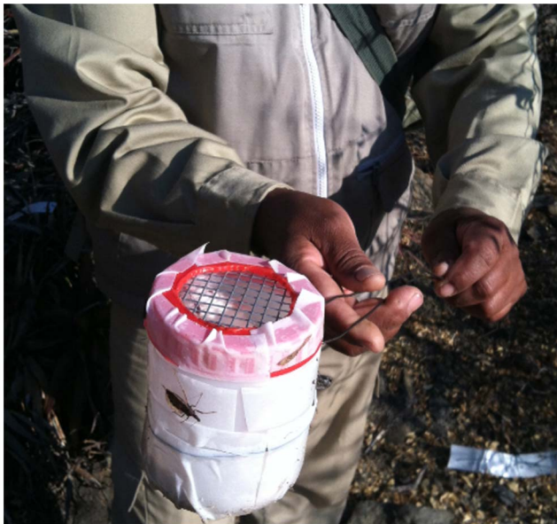
Figure 2. Noireau sylvatic insect vector trap. Traps consisted of plastic containers with a live mouse and wire mesh tops. Double sided sticky tape was placed on the outside of the traps. doi:10.1371/journal.pntd.0003365.g002
