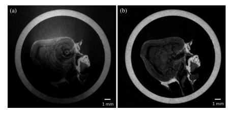
**Fig. 6** CT slices of a rat's heart acquired at the laboratory and processed using (a) the conventional and (b) modified local phase retrieval algorithms. By tracking and correcting for the variation of system parameters over time, severe image artifacts are removed. Adapted with permission from Macmillan Publishers Ltd.: Scientific Reports, Ref. 49, Copyright 2016.
