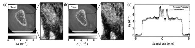
**Fig. 5** Phase tomograms of a chicken bone sample imaged with a conventional x-ray source and retrieved with the (a) reverse projection and (b) conventional EI retrieval algorithms. Scale bars indicate 5 mm. Quantitative values are compared in panel (c), where profiles extracted along the central horizontal lines in the respective tomograms are plotted together. Adapted with permission from IOP Publishing: Journal of Physics D: Applied Physics, Ref. 46, Copyright 2016.
