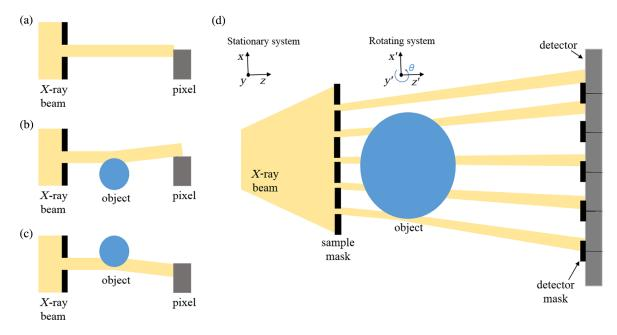
**Fig. 1** (a–c) Schematic diagrams of the synchrotron and (d) laboratory implementations of the EI system. An x-ray beam aligned with the edge of a pixel (a) is refracted away (b) or toward (c) the pixel after passing through an object. In the laboratory, (d) two masks are employed to replicate the EI condition over the entire field of view.
