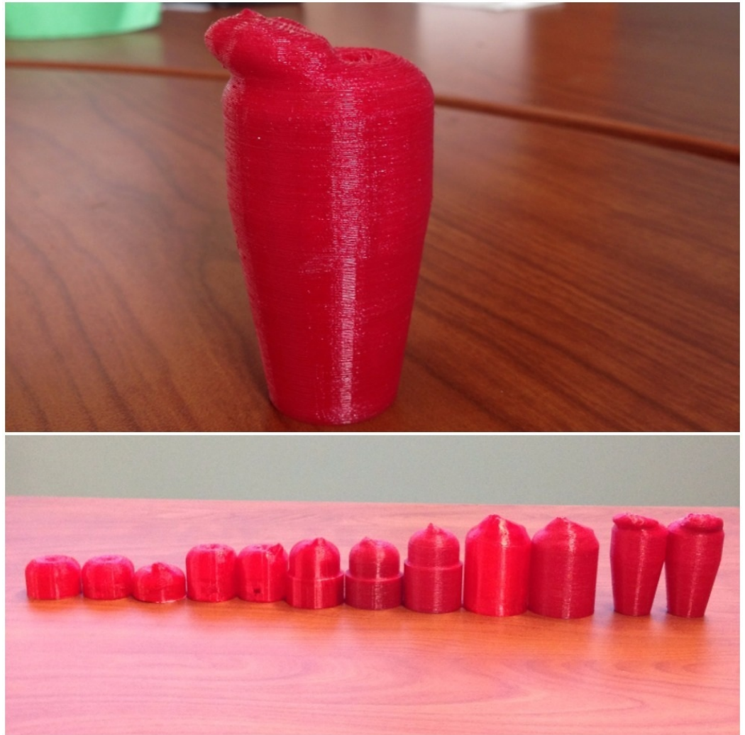
FIGURE 4: Final cervical model with neoplasm made from SemiFlex with the TAZ 6 (top) and evolution of 3D-printed cervical models with PLA, FLX and SemiFlex materials (bottom)
