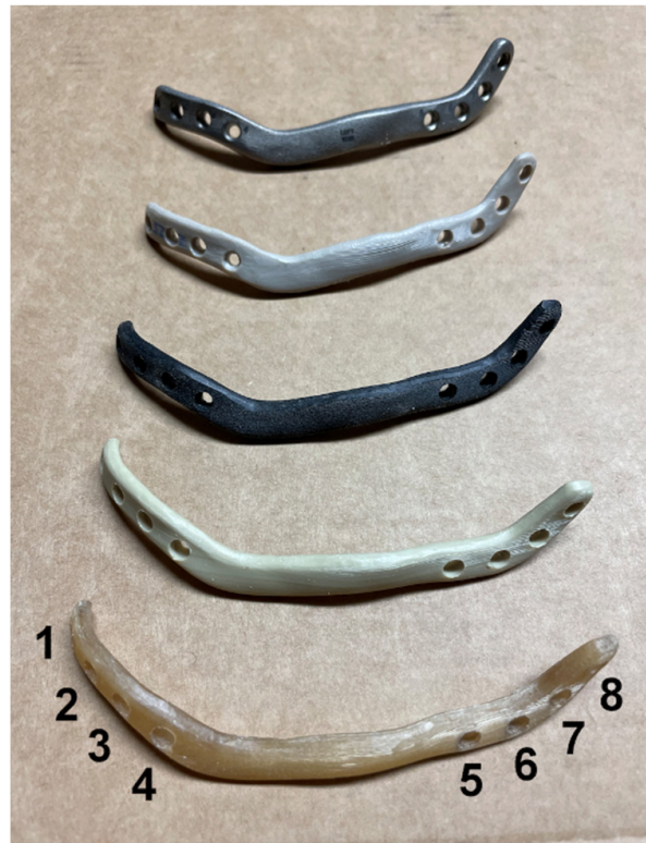
Figure 1. Display of the five different plates used for defect bridging. All plates in this trial are identical in design and dimensions. From top: titanium, polyetheretherketone (PEEK), fiber-reinforced polyetheretherketone (f-PEEK), polyetherketoneketone (PEKK), and polyphenylsulfone (PPSU). The numbers 1–8 symbolize the different drilling holes for implant orientation and selection of the required screw length.
