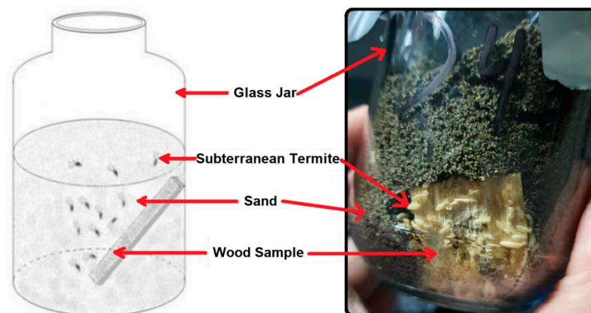
**Figure 2.** Test unit of subterranean termite attack on the wood specimen.
