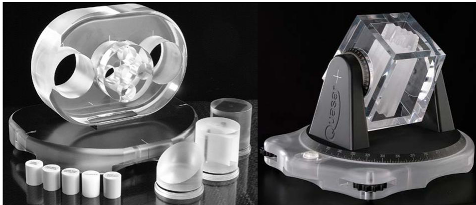
FIG. 1. The Quasar Body Phantom (left) and MLC-Phantom (right) used to test geometrical accuracy of data transferred from Pinnacle to Perspecta.
