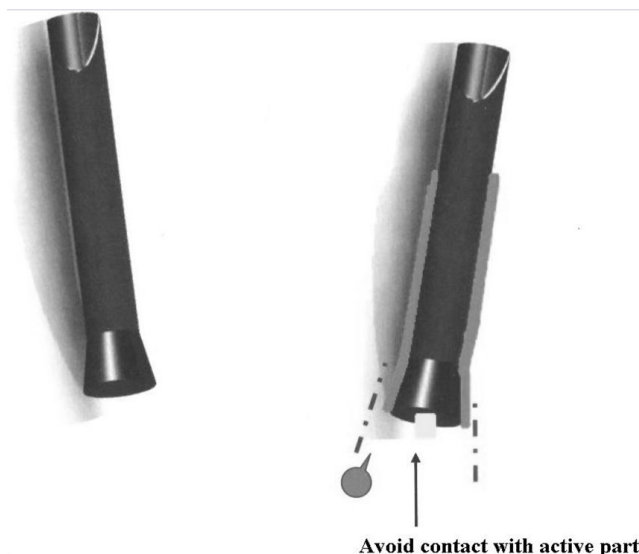
Figure 5 Improvement proposal for the terminal portion of the Roticulator Endo Mini-Shears™.
