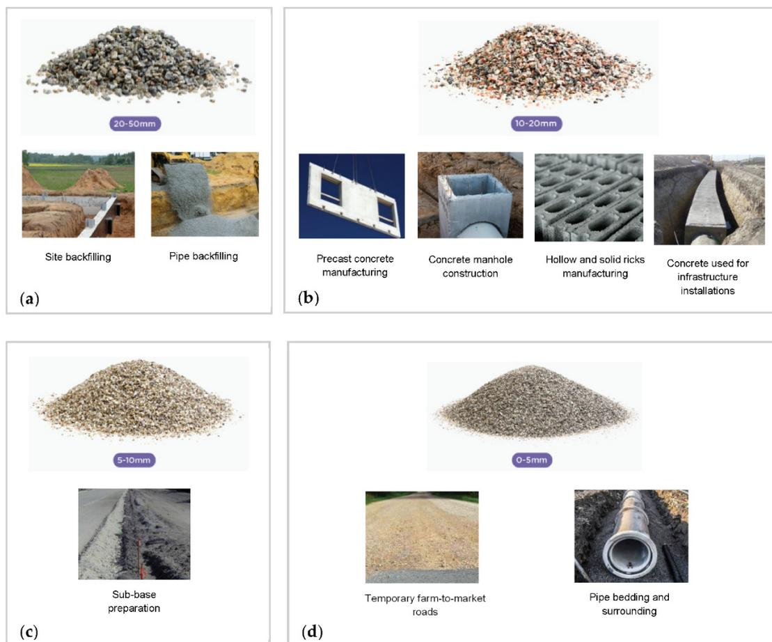
**Figure 8.** Pictorial vignettes of recycled aggregates and their potential uses, (a) 20–50 mm aggregates, (b) 10–20 mm aggregates, (c) 5–10 mm aggregates, and (d) 0–5 mm aggregates. (Source: SIRC [16]).
