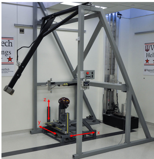
FIGURE 1. The custom impact pendulum device was used to strike a NOCSAE headform mounted on a Hybrid III 50th percentile neck. The head and neck were mounted on a sliding mass that simulates the effective mass of the torso during impact. The slide table has 5 degrees of freedom so that any location on the helmet could be impacted: translation along the x axis, translation along the y axis, translation along the z axis, rotation about the y axis, and rotation about the z axis.
