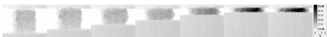
Figure 9. IR images for loading parallel to main fiber orientation (relative density: 0.16). Time interval between consecutive pictures \approx 0.005 s.
