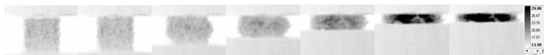
Figure 7. IR images for loading parallel to main fiber orientation (relative density: 0.3). Time interval between consecutive pictures \approx 0.005 s.
