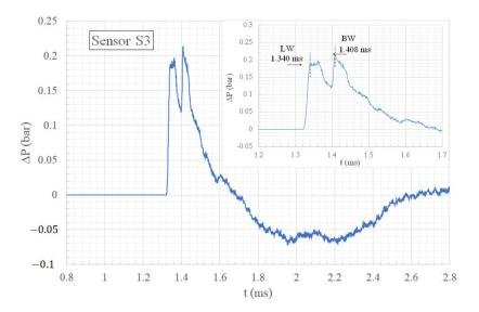
Figure 13. Overpressure time history of sensor S3.
