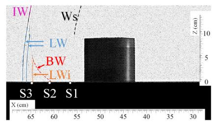
**Figure 12.** Visualization of the shock wave (BW) passing approximately over sensor S3 at t = 1.399 ms. (Ws) secondary shock wave, (LW) lateral shock wave, (BW) bypass shock wave, (LWi) intersection of lateral shock waves.
