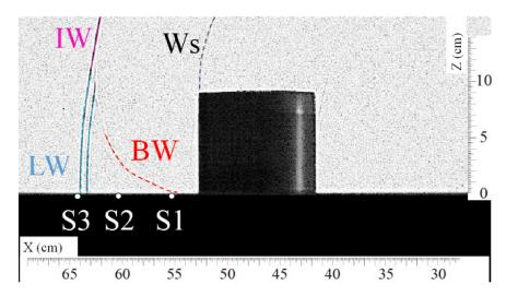
Figure 6. Visualization of the shock wave (BW) passing approximately over sensor S1 at t = 1.257 ms. (Ws) secondary shock wave, (IW) incident shock wave, (LW) lateral shock wave, (BW) bypass shock wave.
