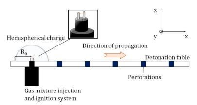
**Figure 1.** Detonation table and ignition device.
