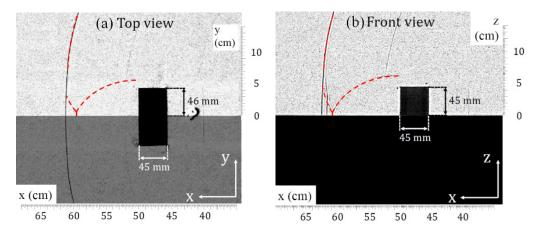
**Figure 14.** Comparison of the bypass wave and the lateral waves downstream of the obstacle Parall-45-92-45. (a) Top view and (b) front view.
