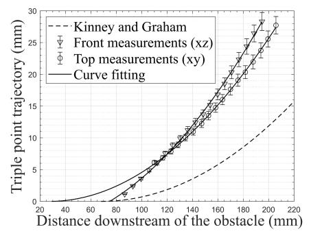
Figure 17. Triple-point trajectory measured downstream of the obstacle Parall-45-92-45 in both directions.
