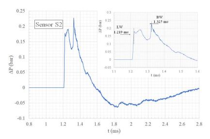
**Figure 10.** Overpressure time history of sensor S2.
