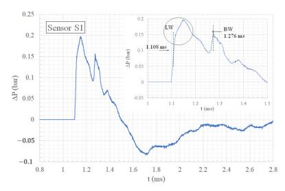
**Figure 7.** Overpressure time history of sensor S1.
