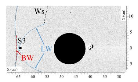
**Figure 11.** Visualization of the shock waves (LW) passing approximately over sensor S3 at t = 1.342 ms. (Ws) secondary shock wave, (LW) lateral shock wave, (BW) bypass shock wave.
