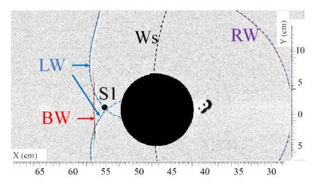
**Figure 5.** Visualization of the shock waves (LW) passing approximately over sensor S1 at t = 1.100 ms. (Ws) secondary shock wave, (RW) reflected shock wave, (LW) lateral shock wave, (BW) bypass shock wave.
