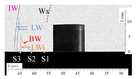
**Figure 9.** Visualization of the shock wave (BW) passing approximately over sensor S2 at t = 1.314 ms. (Ws) secondary shock wave, (IW) incident shock wave, (LW) lateral shock wave, (BW) bypass shock wave, (LWi) intersection of lateral shock waves.
