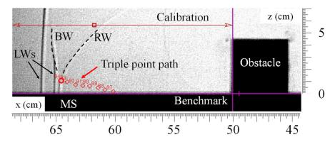
**Figure 15.** Tracking of the triple-point path on Tracker.
