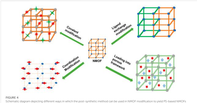
Schematic diagram depicting different ways in which the post-synthetic method can be used in NMOF modification to yield PS-based NMOFs or nanocarrier-based NMOFs.
