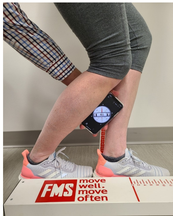
Figure 1: Standing modified lunge ankle DF ROM testing position with inclinometer 2cm below tibial tuberosity.
