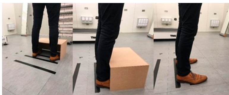
Figure 4. Instructional pictures on methodology for consistent placement of the test person relative to the radiation panel.
