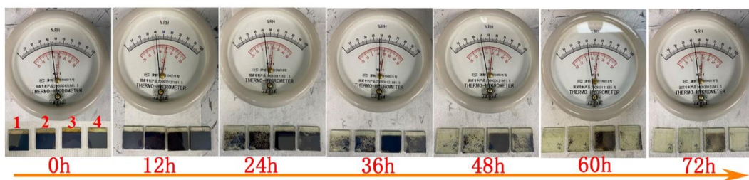
Figure S17. Stability of \text{CsPbI}_{3-x}\text{Br}_x perovskite films with different \text{CdI}_2 concentrations. These films were stored in an environment with a RH between 40% and 50%. (1: reference; 2: 3 mol%; 3: 8 mol%; 4: 13 mol%)
