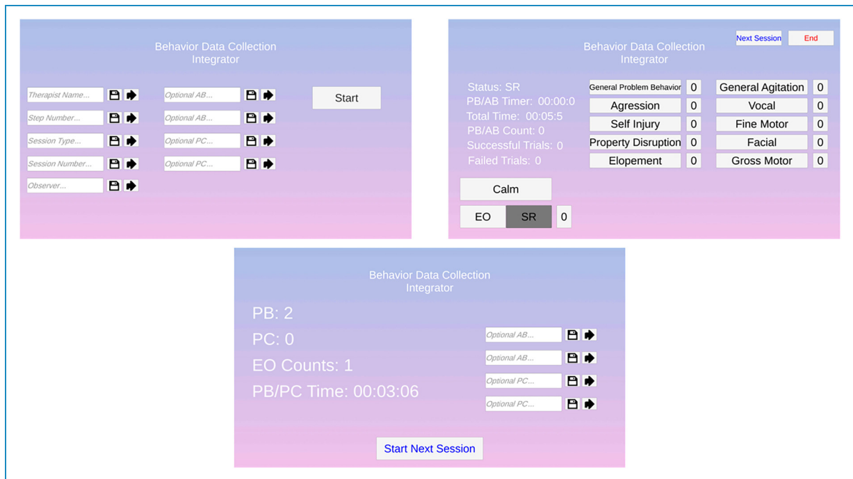
Figure 2. Overview of the behavior assessment application, illustrating its three primary pages: initialization (for entering participant and session details), assessment (for real-time observation and data recording), and summary (displaying session insights postassessment).
