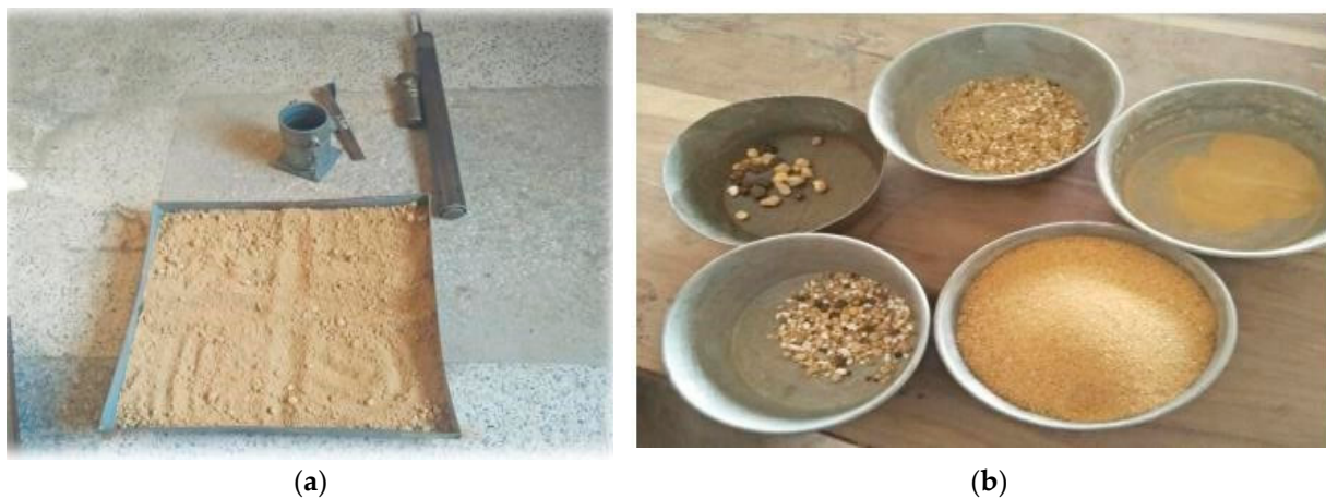
Figure 3. (a) Quartering of representative sample (b) Sieved samples.
