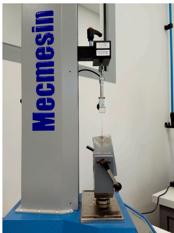
Figure 1. A model mounted in the base handle of the force testing machine.
