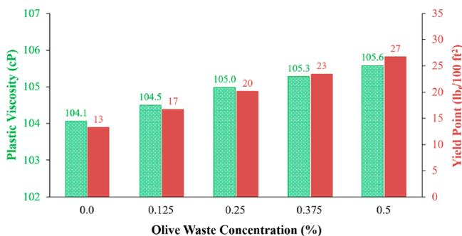
**Figure 2.** Change in plastic viscosity and yield point of the five cement slurries under study.
