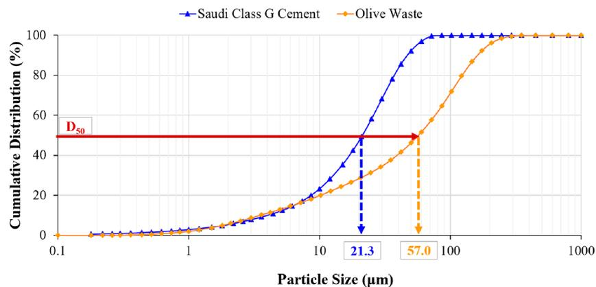
**Figure 1.** Distribution of the particle size of Saudi Class G cement and olive waste.
