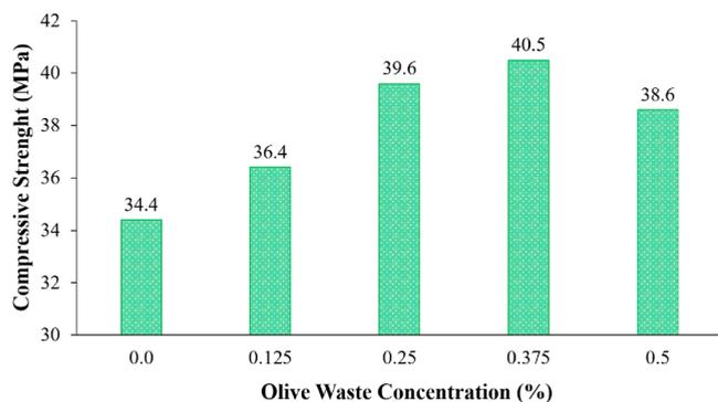
**Figure 5.** Change in the cement matrix compressive strength with the olive waste concentration.
