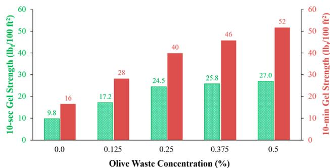
**Figure 3.** Change in the 10 s and 10 min gel strengths of the cement slurries with the olive waste concentration.
