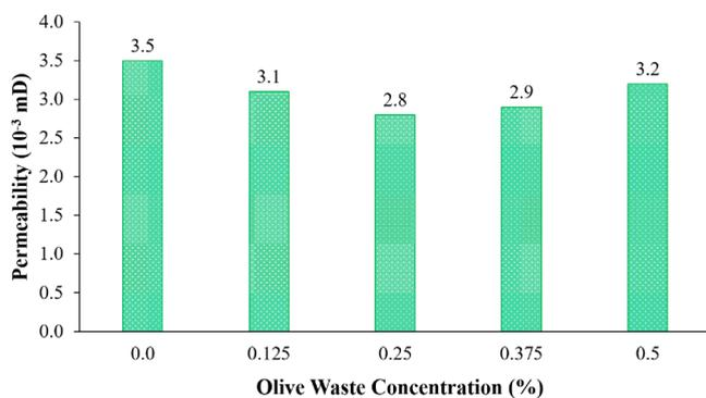
**Figure 6.** Change in the cement matrix permeability with the olive waste concentration.
