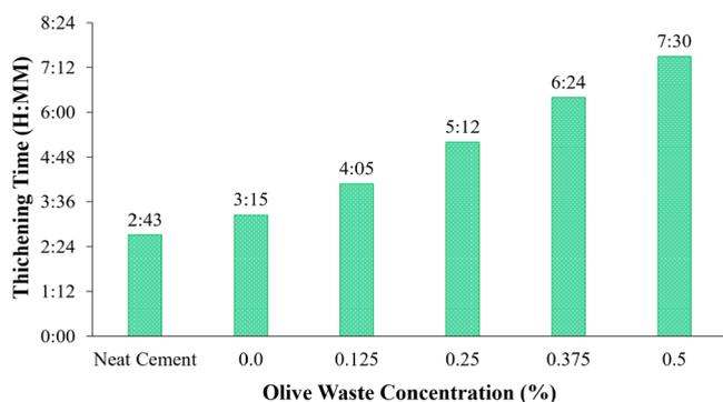
**Figure 4.** Variation of the thickening time with the olive waste concentration. The reported time represents the time needed for every sample to have a consistency of 100 Bc units.
