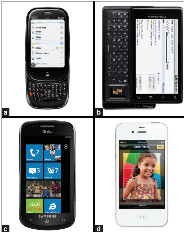
Figure 1: Comparison of modern smartphones (images courtesy Palm, Motorola, Apple, and Samsung). (a) Palm Pre, a vertical slider phone running HP webOS; (b) Motorola Droid, a horizontal slider phone running Google Android; (c) Samsung Focus, a slate phone running Microsoft Windows Phone 7; (D) Apple iPhone 4S, a slate phone running Apple iOS
