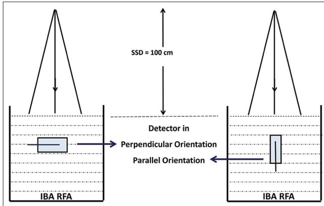
**Figure 1: The schematic representation of detector orientations for the measurement of small field percent depth dose and profile in radiation field analyzer**
