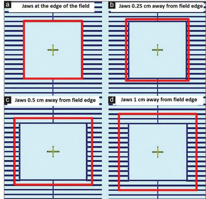
**Figure 2: The configuration of multileaf collimator-defined fields when jaws are positioned (a) close to the edge of multileaf collimator (b) 0.25 cm away (c) 0.5 cm away, and (d) 1.0 cm away from the fields defined by multileaf collimator**
