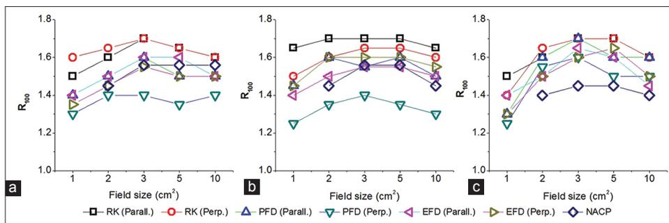
**Figure 4:** The variation in depth of dose maximum acquired with different detectors in parallel and perpendicular orientations for different jaw settings: (a) Jaw alone (b) multileaf collimator alone (c) multileaf collimator when jaw was positioned 0.25 cm away from the field edge
