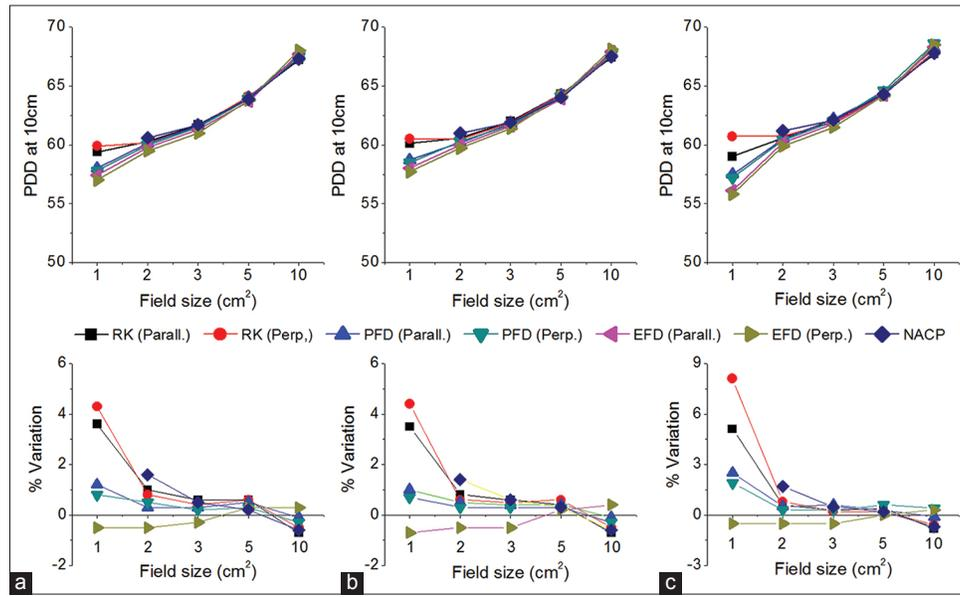
**Figure 3: The variation in dose at 10 cm depth acquired with different detectors for fields defined by (a) jaw alone (b) multileaf collimator alone (c) multileaf collimator when jaw was positioned 0.25 cm away from the field edge**
