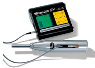
Figure 6. SCHMIDT rebound hammer test apparatus.
