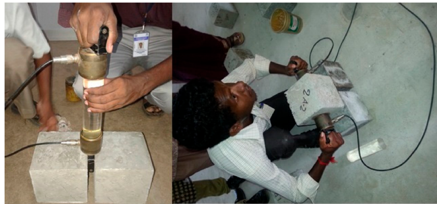
Figure 5. Test set up for ultrasonic pulse velocity test.
