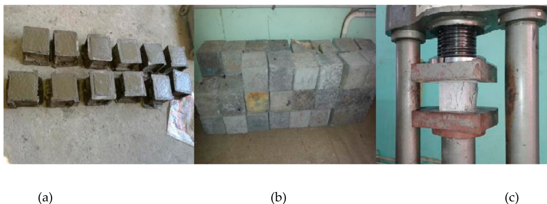
Figure 11. (a) Casting, (b) curing and (c) testing of mortar cubes.
