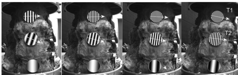
Fig. 16 Direction of movements of individual vertebrates at sample with implant, right bend, direct view
