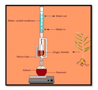
Figure 5. Soxhlet schematic.
