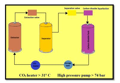
Figure 4. Supercritical fluid extraction using CO<sub>2</sub>.
