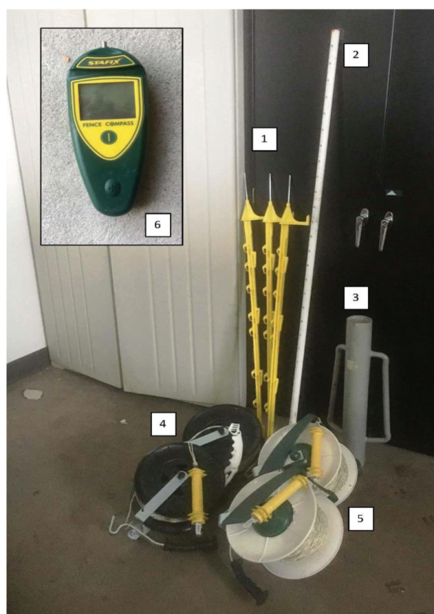
Figure 1. Grazing kit supplied to workshop hosts to promote managed grazing on farms that showcased stockpiling tall fescue including (100) tread-in temporary fence posts (#1); (10) 7/8 in diameter fiberglass posts for use as temporary corners or gate posts (#2); (1) post driver (#3); (2) nongearing fence reels with polywire and handles (#4); (2) gearing fence reels with polywire and handles (#5); and (1) "fault finder" fence tester (#6). Equipment was purchased from Pasture Management Systems (Mt. Pleasant, NC).
