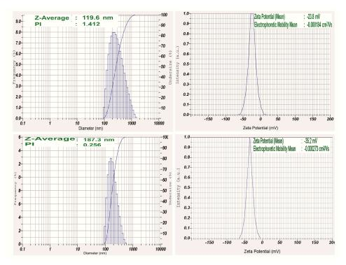
**Figure 1.** Dynamic light scattering (DLS) analysis (mean particle size, polydispersity index and Zeta potential) of poly-lactic-co-glycolic acid nanoparticles (PLGA-NPs) and POL-PLGA-NPs. POL-PLGA-NPs has 187.3 (average size), 0.256 (PDI index), and –23.8 mV of Zeta potential.
