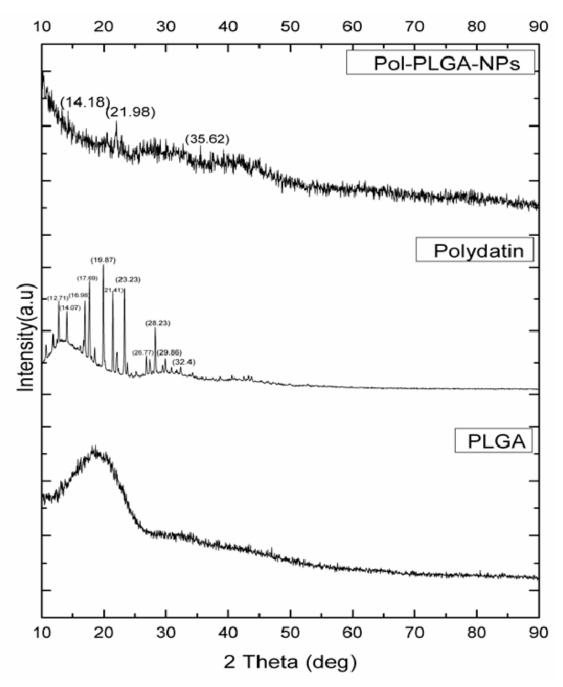
**Figure 5.** XRD pattern of polydatin, PLGA, and POL-PLGA-NPs. POL-PLGA-NPs showings peaks in 14.18°, 21.98°, and 35.62° indicates the entrapment of polydatin in synthesized PLGA nanoparticles.
