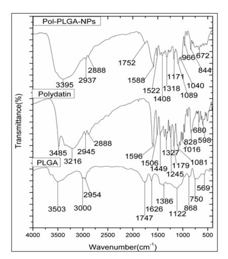
**Figure 4.** FTIR spectrum of polydatin, PLGA and POL-PLGA-NPs. FTIR spectrum of POL-PLGA-NPs showing the peaks of 3503, 3485 cm<sup>-1</sup> shift to a lower frequency at 3395 cm<sup>-1</sup> due to the encapsulation of PLGA.
