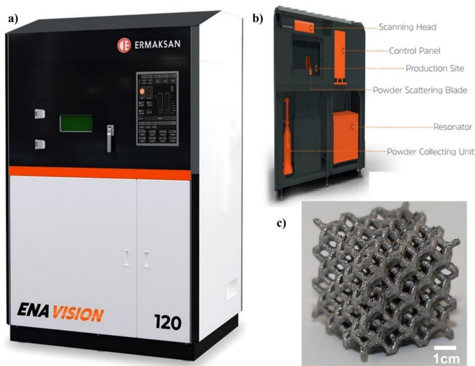
Figure 4. (a) ENAVISION 120 used for validation, (b) machine breakdown, and (c) manufactured specimen.
