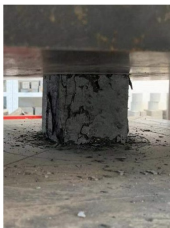
(a) Cubic compressive strength
