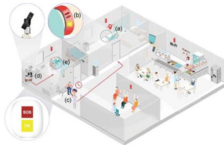
Figure 3. A retirement home (from [20]): heterogeneous sensors can collect data to support the caregivers in their work, while, at the same time, collect valuable data for the indoor localization of both residents and caregivers. The system detects a fallen person through the signal sent by the (a,b) Wi-fi bracelet and alerts (c) the caregiver. The (d) robot assists a (e) bedridden resident requesting help.
