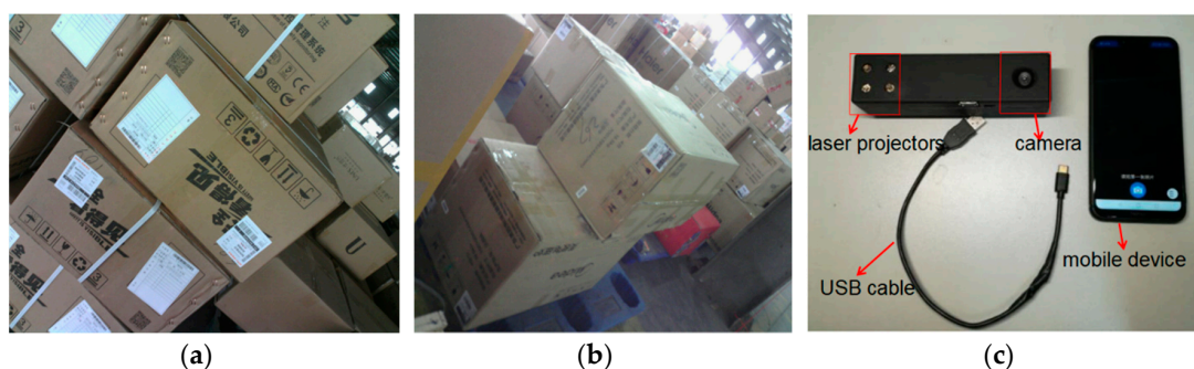
Figure 1. Box in the distribution center and design prototype; (a,b) show the box in the distribution, and (c) shows the proposed system prototype.
