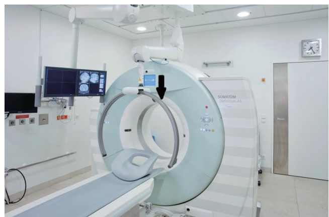
Fig. 1. Laser navigation system (LNS) is fixed to carrying arm attached to computed tomography (CT) room ceiling. C-arm of LNS is positioned in front of gantry (arrow). System does not impair regular use of CT room.
