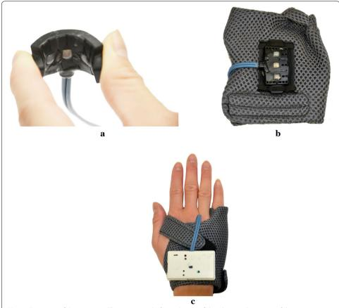
**Fig. 1** Overview of the system. **a** The sensor node. **b** *Inside view* of the glove and position of the sensor. **c** Wearing appearance of the system.
